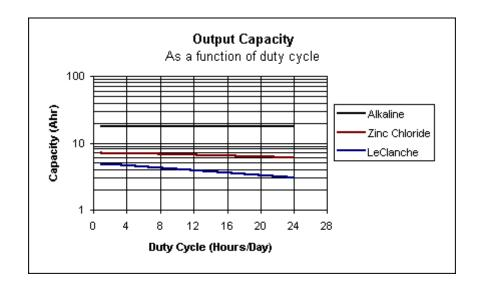
The electrochemical inputs of cylindrical D size batteries typically are in a ratio of 2:3:5 for LeClanche, Zinc Chloride and Alkaline respectively. The differences in efficiency and rate sensitivity between the three systems cause variations in actual output in simulated typical applications as shown in the following table and graph:
