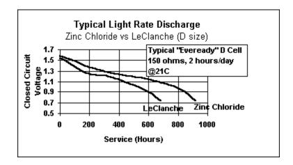
As the drain is increased, the service difference between Alkaline, Zinc Chloride and LeClanche systems increases. This relationship is shown by the following discharge curves. Typical carbon zinc moderate drain is defined as a current that would discharge the cell within 10-50 hours of use at room temperature.
