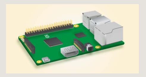
The Raspberry Pi 3 is the third generation Raspberry Pi. It replaced the Raspberry Pi 2 Model B in February 2016. Compared to the Raspberry Pi 2 it has:
