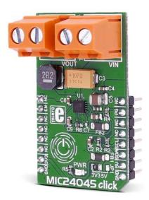
**MIC24045 click** carries MIC24045 I2C-programmable, high-efficiency, wide input range, 5A synchronous step-down regulator from Microchip. The click is designed to run on either 3.3V or 5V power supply. It communicates with the target microcontroller over I2C interface with additional functionality provided by the following pins on the mikroBUS<sup>TM</sup> line: RST, INT.
