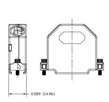
MATERIAL: DIE-CAST ZINC ALLOY PLATING: NICKEL OVER COPPER JACKSCREWS: STEEL, ZINC PLATED STEEL, ZINC PLATED STEEL, ZINC PLATED STEAL, ZINC PLATED STEAL, ZINC PLATED STEAL, ZINC PLATED STEEL, ZINC PLATED
