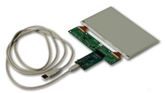
Figure 2.3: USB2TCM\_v1.1 interface connected to a TCM-P74
