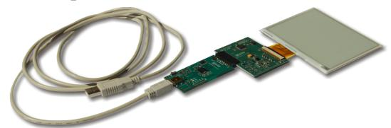
Figure 2.2: USB2TCM\_v1.1 connected to a TCM-P441
