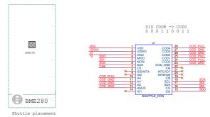
BME280 shuttle board electrical layout
