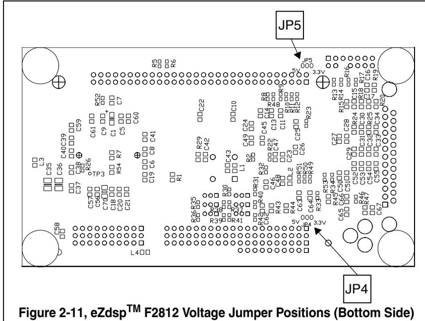
Figure 2-11, eZdsp™ F2812 Voltage Jumper Positions (Bottom Side)
