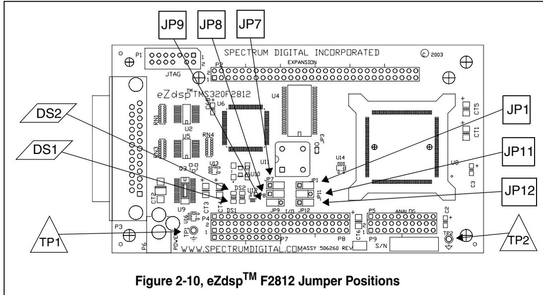
Figure 2-10, eZdsp™ F2812 Jumper Positions
