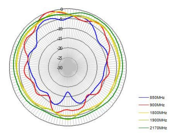
B. Radiation Pattern, Aligned at the Connector
