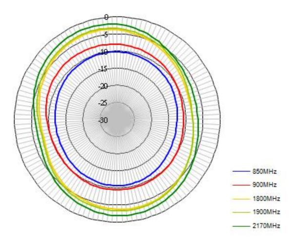
A. Radiation Pattern, Azimuth Plane (XY)
